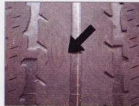
Worn out tyre treads that should be replaced
