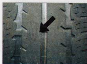
Worn out tyre treads that should be replaced
